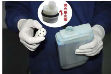
Clocking/(proper positioning) of (insert valve. Proper tightening of retainer cap to provide good seal.
