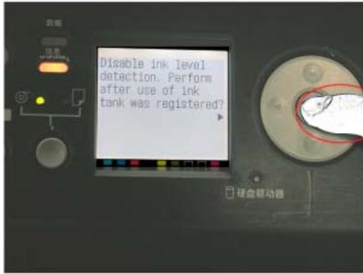
(19)Warning: Disable ink level detection. Perform after use of ink tank was registered. Press OK.
