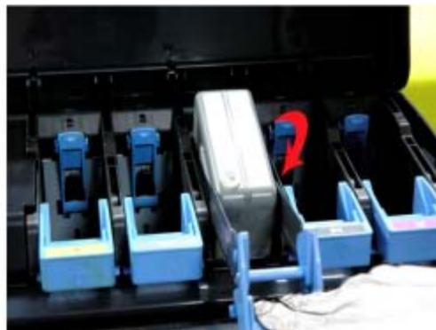
(4) Remove the ink tank holding grip and press OK. Put back the refilled cartridge to the printer.
