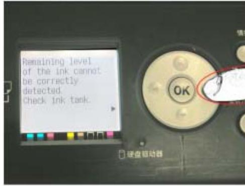
(6) Alarm: Remaining level of the ink cannot be correctly detected. Check ink tank. Press continue.
