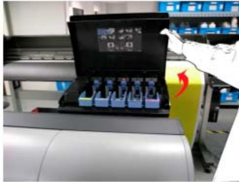
(2) Lift ink tank lock lever until it stops and push it down.
